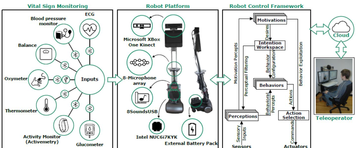
Figure 1: Enhancing a beam+ Telepresence Robot for Remote Home Care Applications
